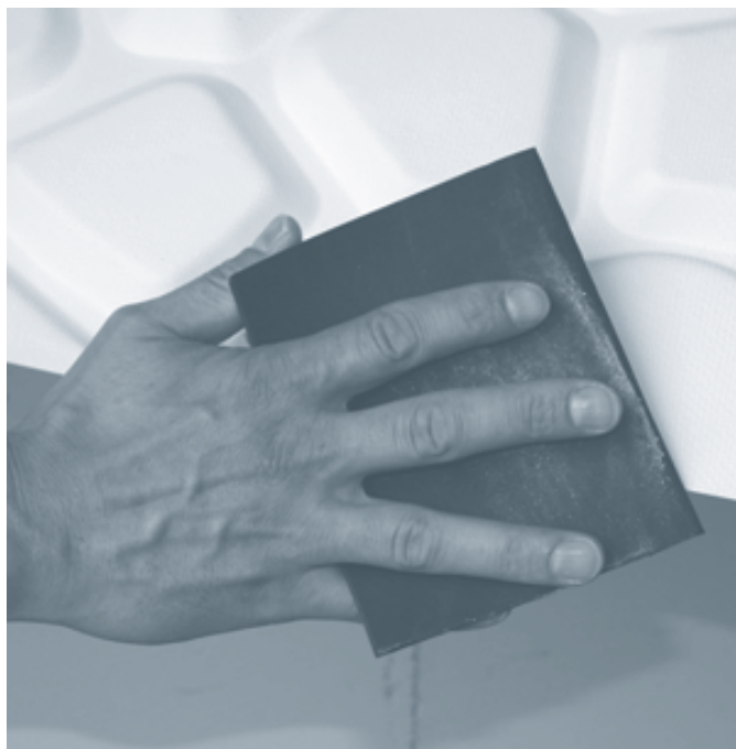
Sand the cut edge to a smooth finish.
